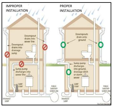
Clean-water connections come from four primary sources that are improperly installed: *sump pumps, exterior floor drains, exterior foundation drains, and roof drains*.
